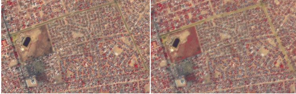
Figure 11 : Angle of incidence impact on Spot-6 1,5 m images in a dense urban area (subvertical image on the left and high angle of incidence image on the right)
