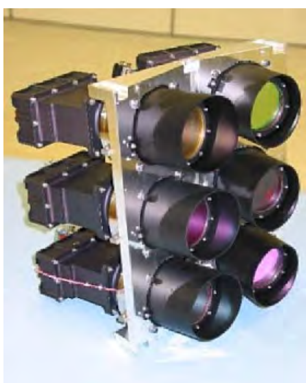
Figure 1-2: SSTL SLIM6 Imager on KazSTSAT
