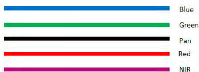
Figure 1-4: ALSAT-1B sensor band arrangement on one CCD
