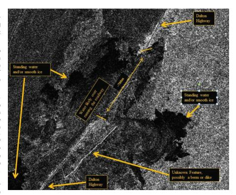
collect and delivery a 1.25m StripMap image to AKDOT & PF in less than 18 hours of the original request. AKDOT & PF immediately used the radar image to assess the flooding impact along the Highway, in particular to identify washed
