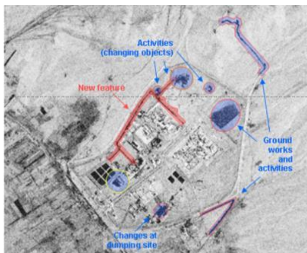
Figure 2: TerraSAR-X Sample for Coherence Change Detection at Iranian Heavy Water Research Reactor in Arak, Iran
